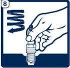
Screw in spark plug by hand as far as possible, without tightening it
