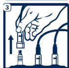
Disconnect ignition cable or ignition coil
